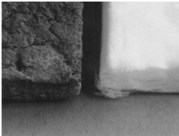
FIGURE 10.9 Photograph of the pads used in a counter diffusive radiant heater. On the left is a pad impregnated with catalyst, and on the right is an insulation pad.
